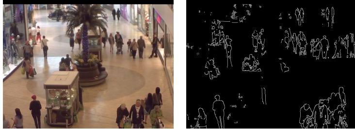
Figure 7: The edges of the foreground, as detected by the Canny algorithm.
