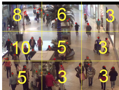
Figure 2: Locality can be introduced by grid cell-based subdivision. The number of reference points (heads) is displayed for each cell.
